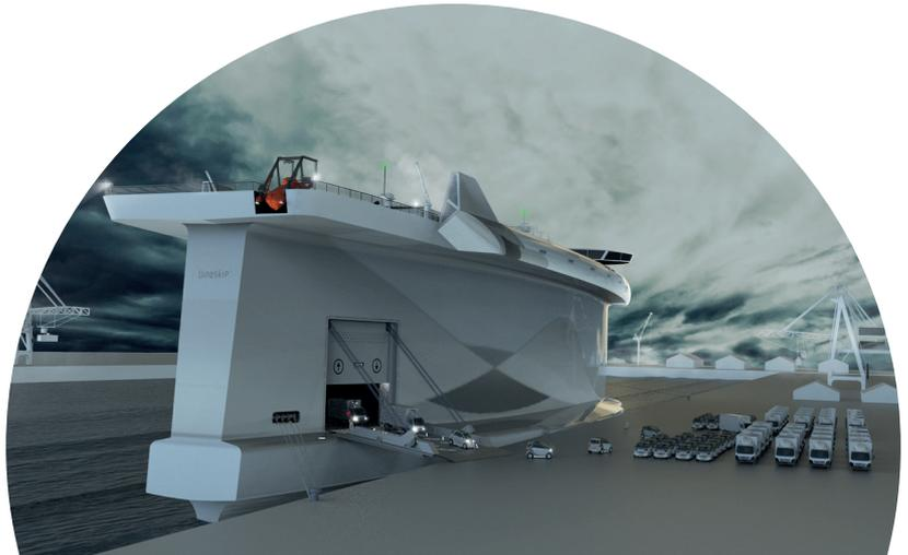
The kind of cargo transported also plays a key role in the viability of wind propulsion systems onboard. While on a route from Brazil to China with iron ore, for example, where speed plays a small role, a design like this would work well. On shipping services where higher speed is essential (minimum 14 knots), however, sail-assisted ships might not be an efficient option, which is the case with maritime transportation of vehicles across the Atlantic.
